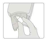
2 Place microcuvette into analyzer.
