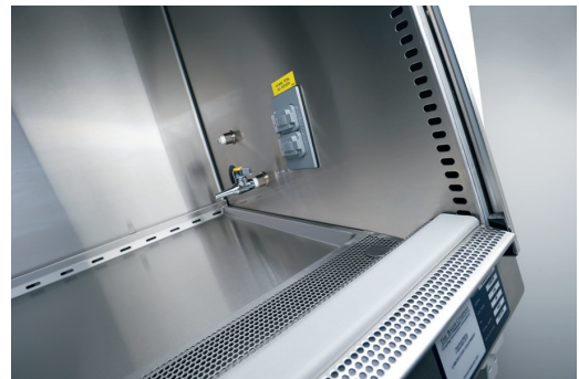
High-velocity return air slots maximize protection.
