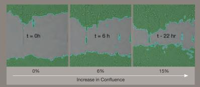
In a wound healing migration assay, a wound is produced on a fully confluent cell layer by a mechanical tool or generated by a device inhibiting cell growth in a defined area. Celigo is used to image the entire well with a wound at multiple time points. Confluence is automatically calculated for each well. The increase of confluence is obtained for conditions which enhance cell migration.
