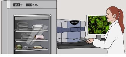
High resolution bright field whole-well imaging and direct cell counting takes about 5 minutes or less for a 96- or 384-well plate.
