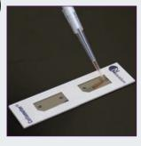
Pipette 20 µl of Cell Sample
